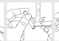
Use needle or brush hair to clean Assemble the steam tube the small hole of side nozzle.
