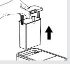
Use the integrated handle on the lid to lift the water tank.
