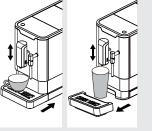
Place a cup under the coffee spout, adjust the position of the coffee spout or remove the drip tray to suit different sizes of cup.
