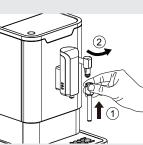
Assemble the steam nozzle to the appliance.
