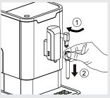
Disassemble the nozzle by rotating counterclockwise and pulling downwards.
